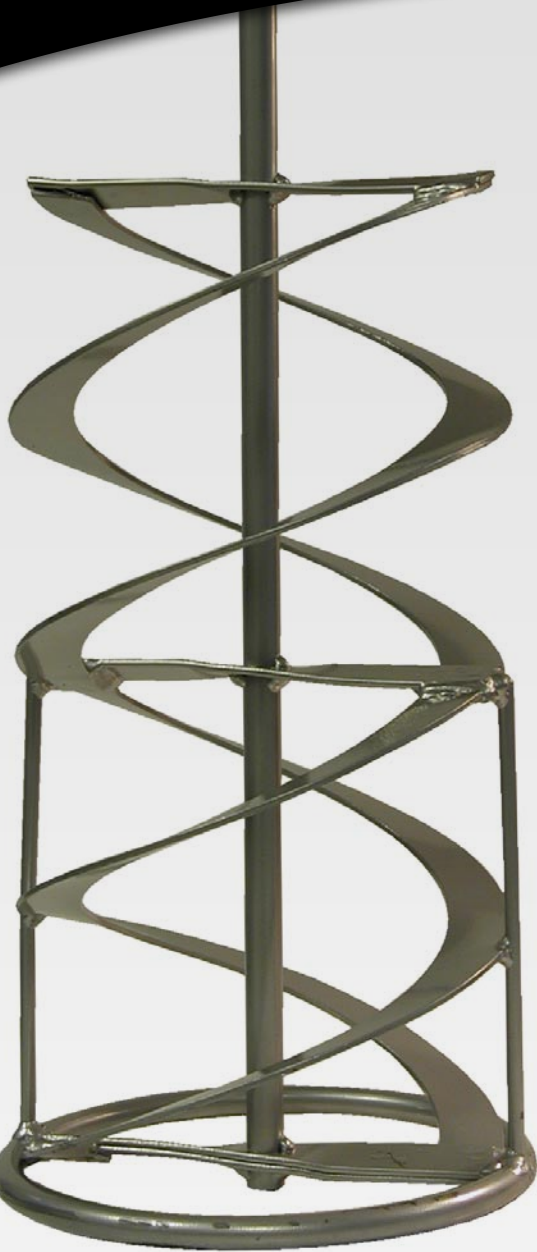
Shown: WMP-TWD mixing paddle. Mixes material from the bottom up while the shear bars provide proper color mixing.
