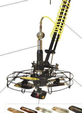
**BLADES**With the HoverTrowel's blade selection you can power trowel systems normally hand troweled. The HoverTrowel has various blade types ranging from standard tool steel, stainless steel, a line of floats like mahogany, laminated resin, magnesium, and other specialty blades.
